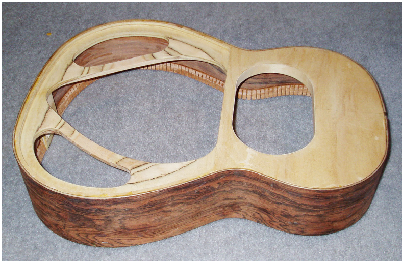
Fig. 3: Guitar carcass, showing laminated skeleton reinforcement for the sides.
