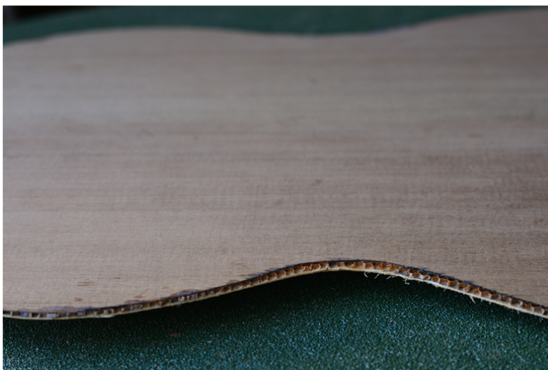
Fig. 4: Laminate soundboard of Nomex core and solid wood 'skins'
