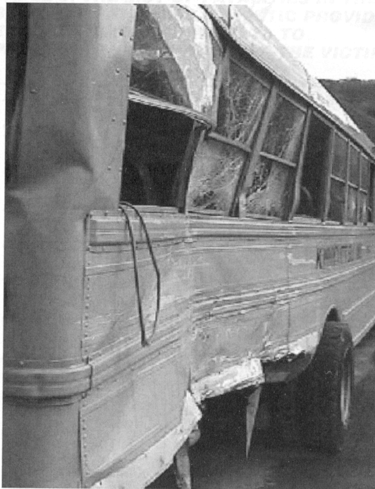
Figure 1. Exterior crush damage of school bus.
